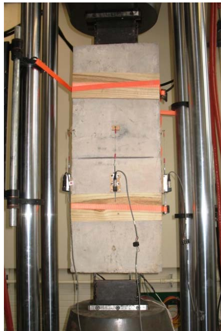
Figure 4-29: Saw-Cut Specimen in MTS Machine
