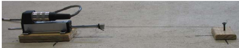
Figure 4-6: Linear Potentiometer on CIP Slab across Expected Crack Location
