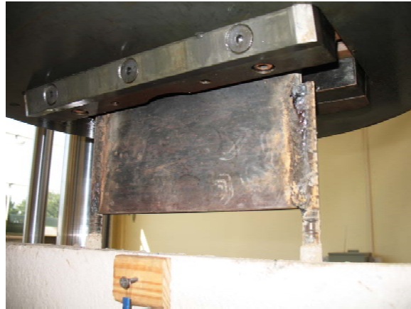
Figure 4-23: Welded Plates in MTS Grip
